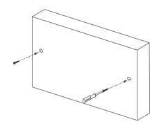
4 Secure the wall mount bracket onto the main unit with 2 supplied screws.
